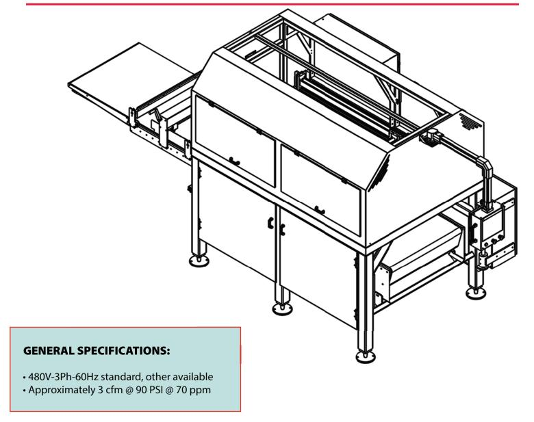
**Optional AutoEye** technology utilizes a high-resolution camera. The optical recognition identifies the position of incoming packages. This allows for proper orientation prior to pattern forming, with the ability to correct mis-aligned or rotated packages.
