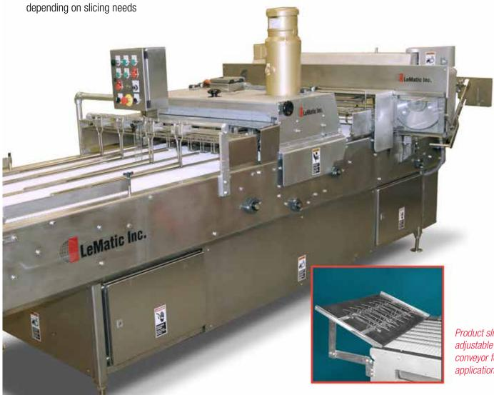
Product slide with adjustable guide for conveyor feed applications
